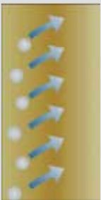
Slowly soluble salts dissolve and migrate towards the surface as the stone dries
