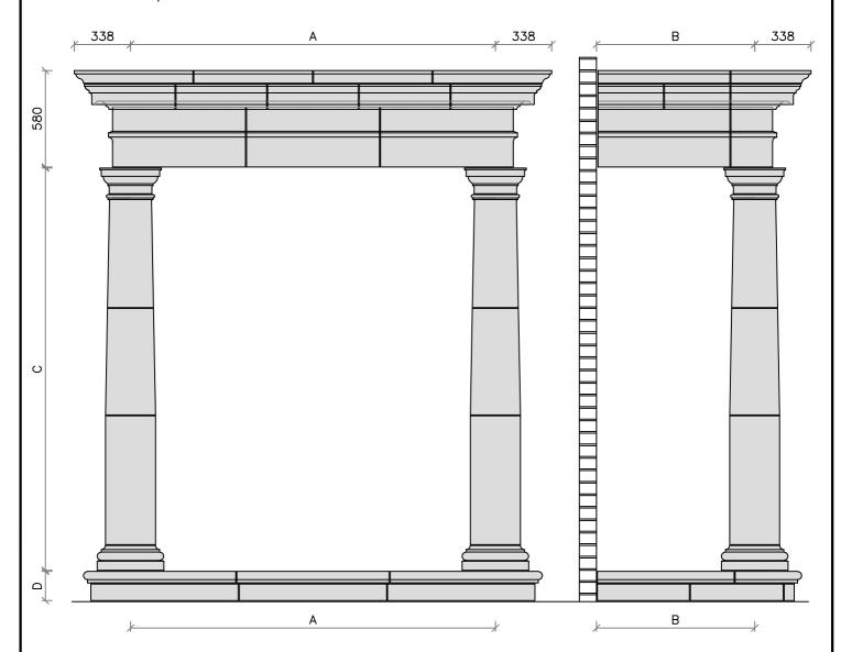
Dimension A is centre line of column to centre line of column
