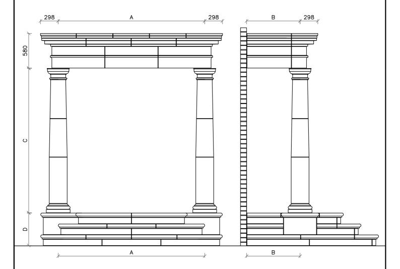
Dimension A is centre line of column to centre line of column
