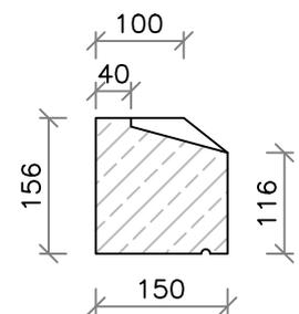
Max length of C1R units are 600mm and C2R to C5R units are 1200mm. Longer units will be manufactured in manageable pieces to suit.
