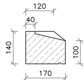
Max length of C1S units are 600mm and C2S to C4S units are 1200mm. Longer units will be manufactured in manageable pieces to suit.
