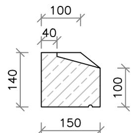
Max length of C1-Imp units are 600mm and C2-Imp to C5-Imp units are 1200mm. Longer units will be manufactured in manageable pieces to suit.
